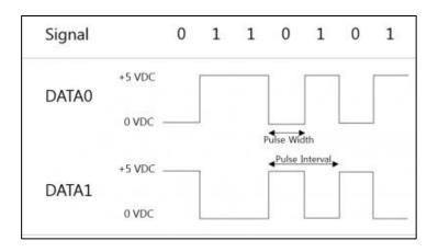
Traditional Wiegand cards generally possessed 26 bits of data. These bits consisted of two error checking bits, 8 facility bits, and 16 ID bits. The facility bits would be used to specify which sub location at an establishment was being accessed (e.g. storage room vs. classroom). The ID bits would contain the actual combination of bits that would provide access into the desired location.
